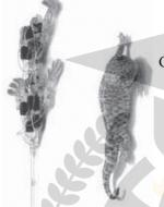
G Stickybot now walks up vertical surfaces of glass, plastic, and glazed ceramic tile, though it will be some time before it can keep up with a gecko. For the moment it can walk only on smooth surfaces, at a mere four centimeters per second, a fraction of the speed of its biological role model. The dry adhesive on Stickybot's toes isn't self-cleaning like the lizard's either, so it rapidly clogs with dirt. "There are a lot of
